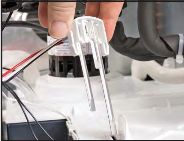
1. Remove Water Level Sensor
