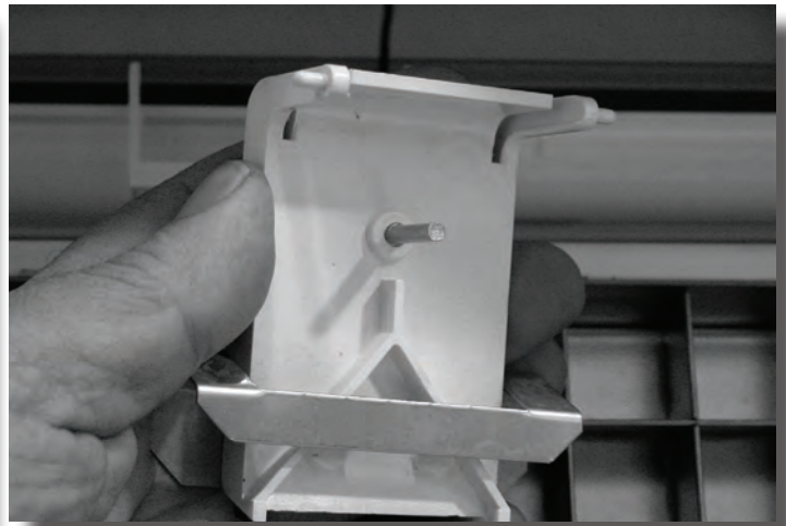
11. Separate parts, clean with diluted scale remover, rinse with clean water, blow dry and reassemble. (See page 5)
