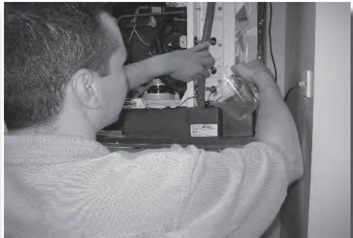
17. Wait until display code blinks 'A d 1', then add the sanitizer solution into reservoir.
